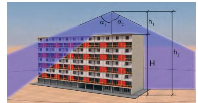
Fig. 7 – Protection volume angles \alpha_1 and \alpha_2 depending on heights h_1 and h_2 .
