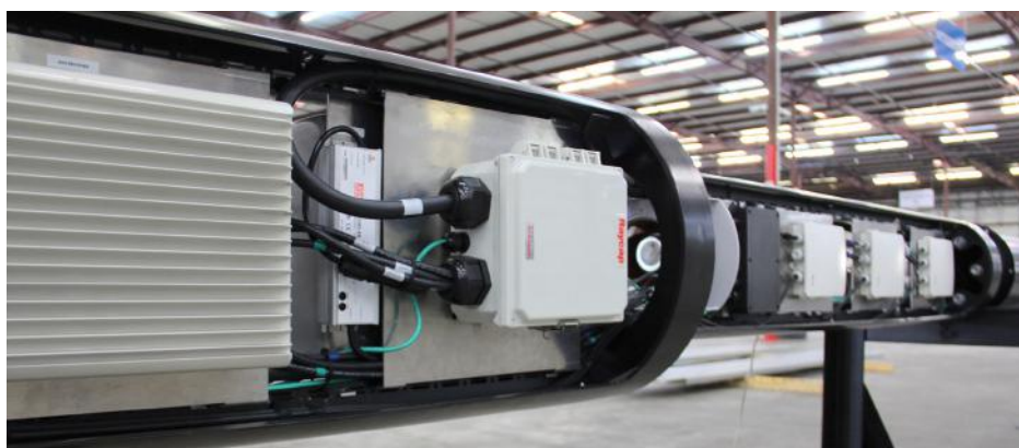
Figure 1: AC power and equipment compartments in an integrated 5G small cell pole assembly.
