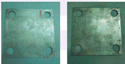
b) plates with galvanic zinc coating after removing the corrosion of the zinc coating
