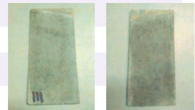
b) plates with thermal diffusion zinc coating after removing the corrosion of the zinc coating
