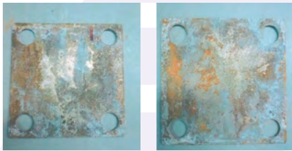
a) plates with galvanic zinc coating
