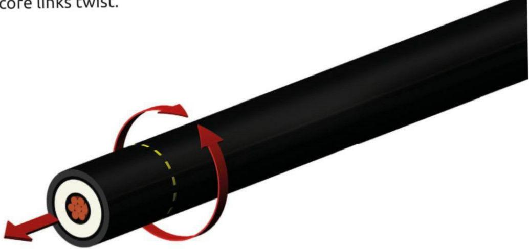
Use wire debarking machine to remove the two outer cable sheath at a distance of 120mm. Wire debarking machine should be properly set to avoid damage to cross-linked polyethylene insulation film.
