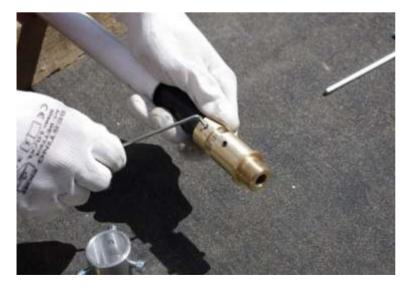
3. Coat the threads of two screws with glue, then put them in the holes and tighten to the brass connector.
