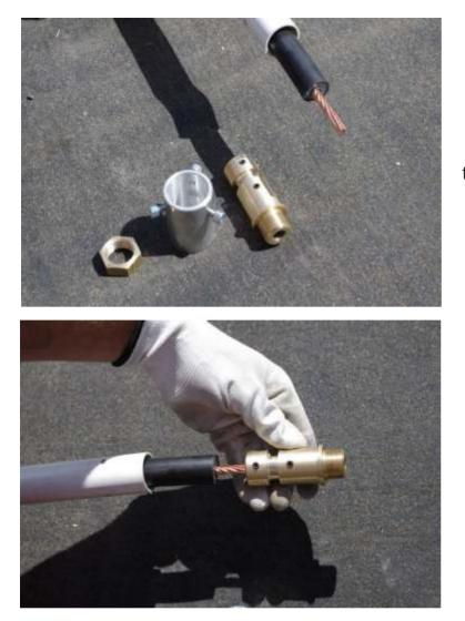
1. Place high voltage insulated cable in the insulation bar.
