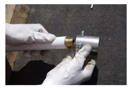
5. Put the insulating bar tip on to the brass connector, so the brass thread is visible.
