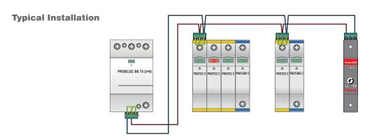
ProALARM is a failure indication device that informs a user of the need to replace a failed SPD. It can be quickly and easily installed next to the SPD on the same rail, and by making connection between the RC contacts of the SPD and the unit.
